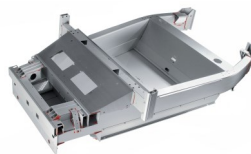
Adhesively bonded aluminium chassis of the Lotus Elise
