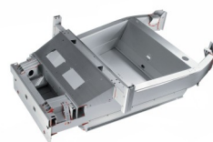
Bonded Aluminum chassis of the Lotus Elise Source: Group Lotus PLC
