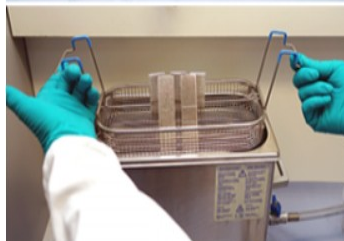
Surface cleaning in an ultrasonic IPA bath in the fume hood
